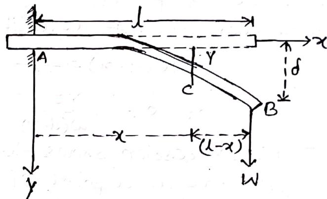
Let us consider a thin, uniform and light beam of length  $l$  clamped horizontally at one end  $A$ . When it is loaded with a weight  $W$  at the free end  $B$ , the end  $B$  is depressed downward compared to  $A$  so that the beam undergoes bending. Since the beam is light, the whole depression may be taken as due to the load  $W$ .
